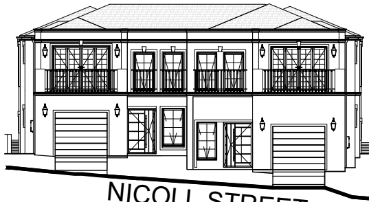
2 SOUTH WEST ELEVATION 1 : 250
